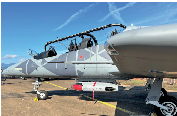
360° Radar-Modular Design; Radar SCAR-Pod on De Havilland Twin Otter; Radar SCAR-Pod on L39NG
