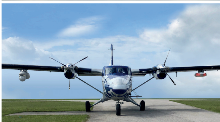
Radar SCAR-Pod with 240° coverage; Guardian 400 Twin Otter with EO/IR and Radar SCAR-Pod
