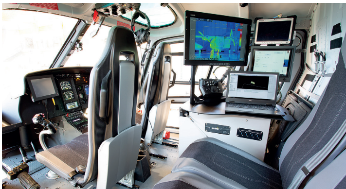
AS350 with 3 sensor positions; Operator workstation
