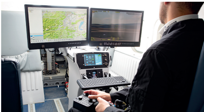
Twin Otter Guardian 400; Airborne LINX Operator Workstation
